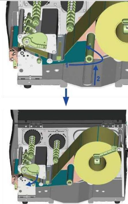
12. Close the printer cover to complete installation of the dispenser.
