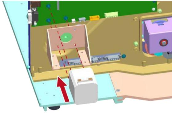
7. Fix the motor module on the base of the printer.
