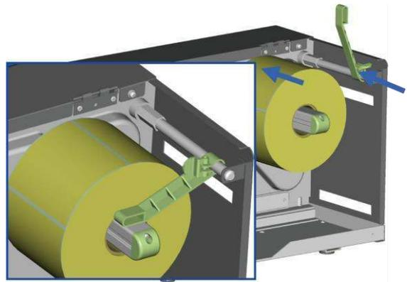
7. Load the label roll into the printer as shown in the illustration.
