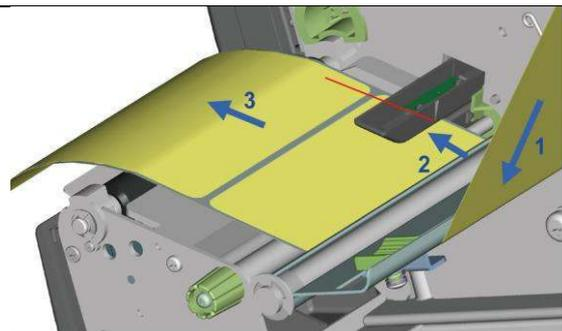
9. The labels pass between the wall of the printer housing and the adjustable paper guide.
