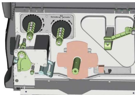
※After the rewinder module is installed, please send the command "`^XSET,REWINDER,1`"、"`^O1`" through Golabel to activate the rewinder module.
