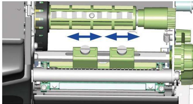
4. Turning the screw clockwise increases the pressure, while turning it anticlockwise reduces the pressure.
