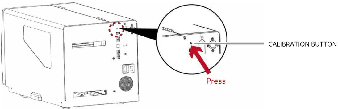
Press C-button for 2 seconds, it will make an auto-sensing to calibrate the label and ribbon's parameters.
