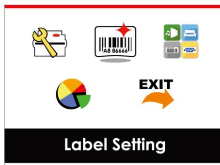
On MAIN PAGE, select the "EXIT" icon and press the FEED button to exit from SETTING MODE and the printer goes back to READY status.
