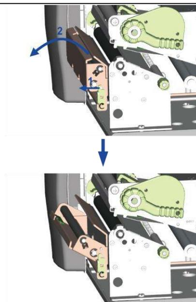
8. Pass the label liner through the print mechanism and from the bottom up onto the rewinder (as in arrow 1 Shown).
