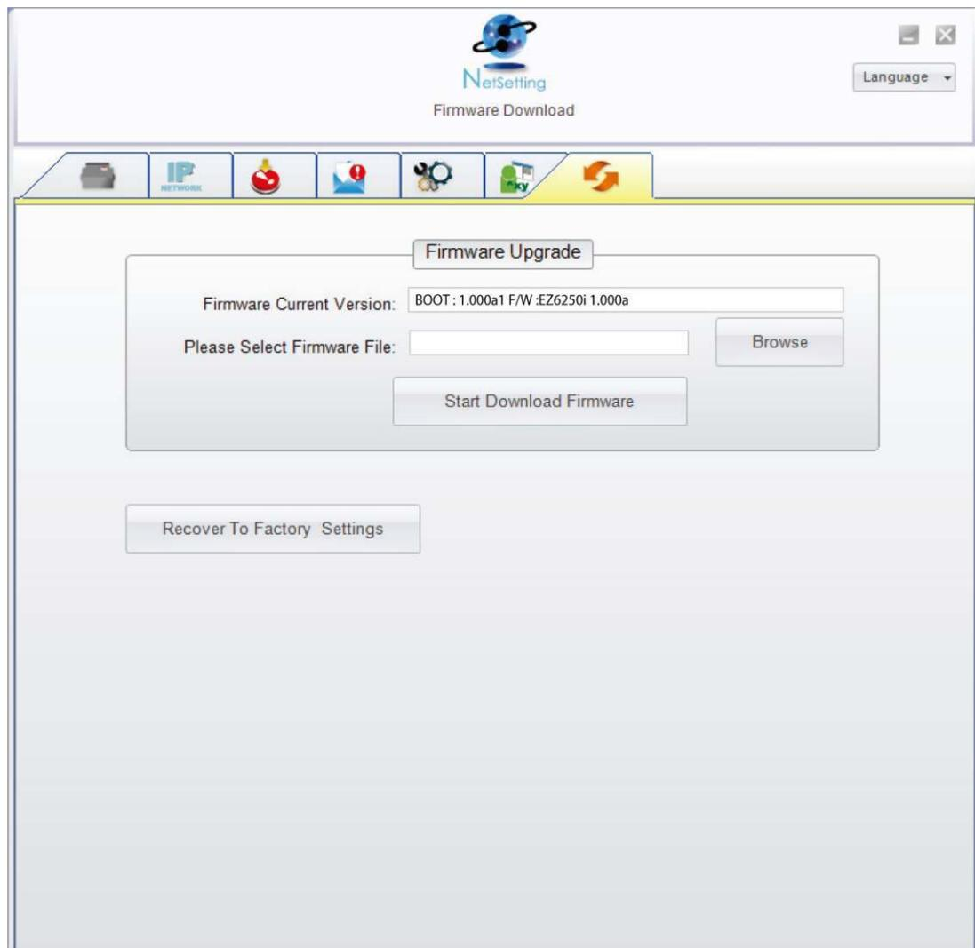
In addition to the firmware update, you can press “Recover To Factory Settings” button to restore the printer configurations back to factory default.
