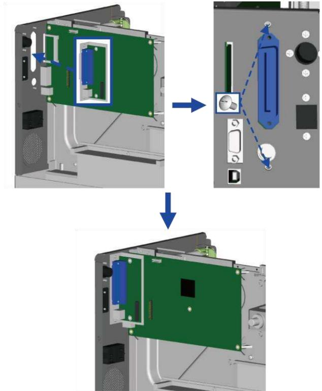
5. Connect the 30-pin connection cable to the motherboard.
