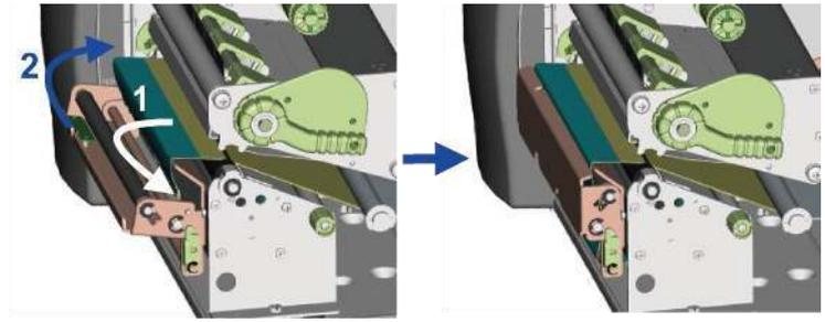
10. Wind the label liner around the rewinder and secure it using the retention clip.
