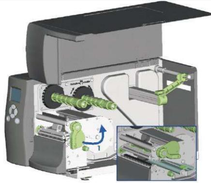
When using a variety of label stock and ribbons, the ink may not be evenly distributed. If there is no printed image on one side of the paper, or the ribbon wrinkles, the print head pressure must be readjusted using the TPH spring boxes.
