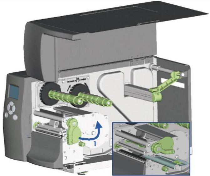
3. Pull the release catch for the label roll guide to the right as shown by the blue arrow 1.
