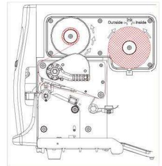
5. Pass the ribbon under the print head and back up on the other side. Attach it to the empty ribbon core.
