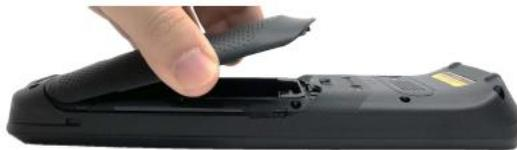
3. Press down the battery cover to secure in place. Make sure there is no gap between the device and the battery cover.
