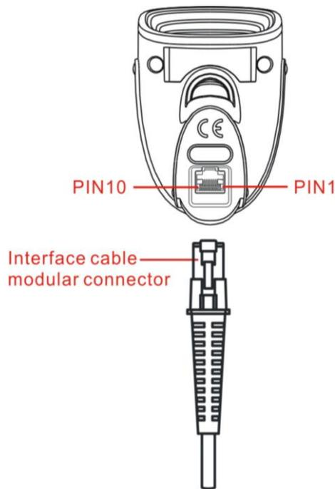
Figure 2-2 Cable connector interface pin-outs
