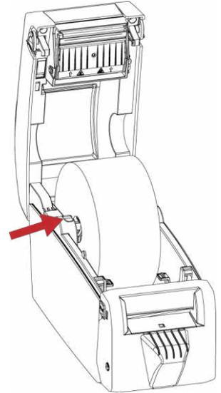
6. Pass the label under the paper guides and pull it forward.
