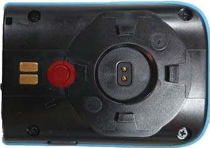
Step 2. Align the four grooves from the trigger module with MS652Plus, also make sure arrows from both sides are close together. Please adjust the arrow alignment as shown in the photo below.
