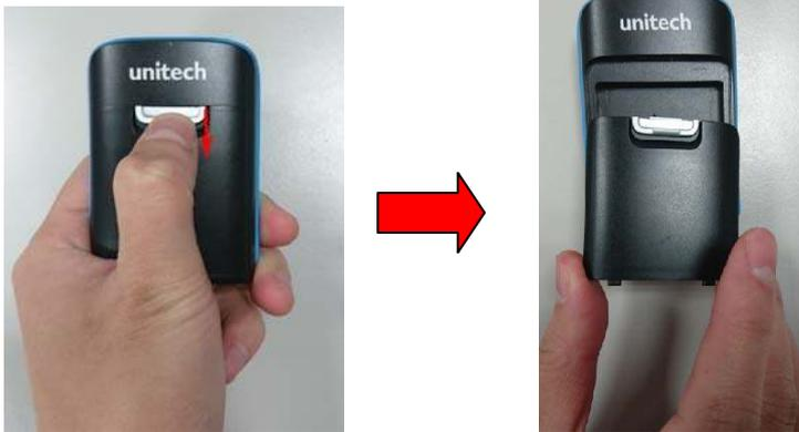
Step 2 : To install the battery, slide the battery and press down the battery to secure it until you hear the clicking sound.
