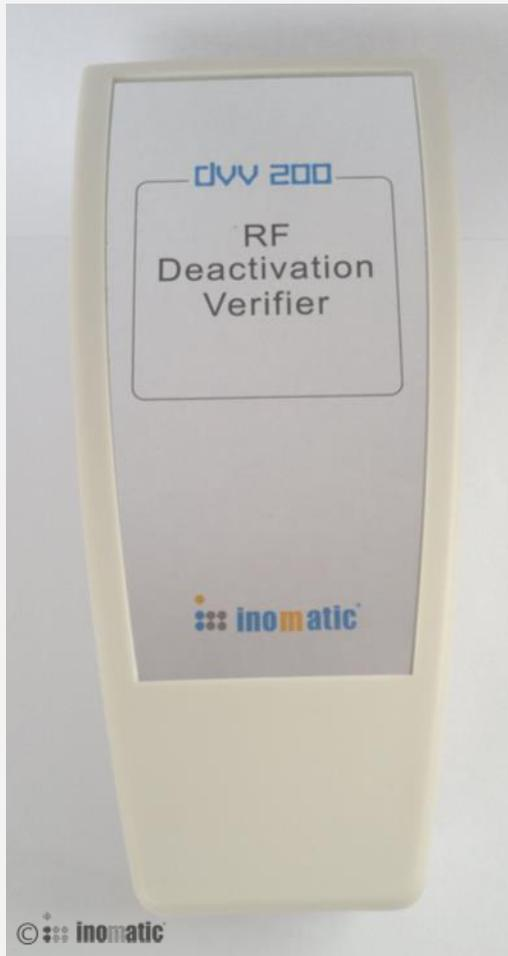
*The Deactivation Verifier DVV-200 allows easy checking of the deactivation height of the deactivator. It works on a frequency of 8.2MHz. A built-in buzzer and LED indicate the effective working height of the deactivator. The device is very useful for a quick check of the deactivator.*
