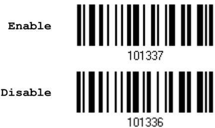
Decide whether to enable EAN-13 378/379 Addon Mode. When enabled, barcodes starting with 378/379 won't be decoded if the scanned barcodes do not have the Addon 2 or Addon 5 suffix.
