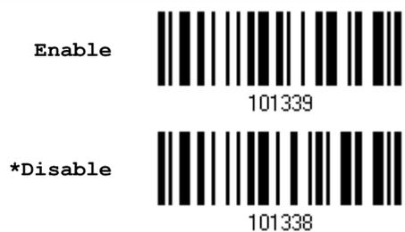
Decide whether to enable EAN-13 977 Addon Mode. When enabled, barcodes starting with 977 won't be decoded if the scanned barcodes do not have the Addon 2 or Addon 5 suffix.
