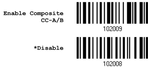
Decide whether to enable GS1 formatting for Composite CC-A/B. When enabled, the field separator and application ID mark will be automatically added to the output data.
