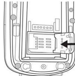
5. Close the cover over the slot, and then slide the cover to the left to lock the SIM card.
