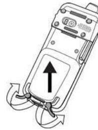
**NOTE:** Make sure the battery compartment cover is securely closed, or you may be unable to turn ON the terminal.
