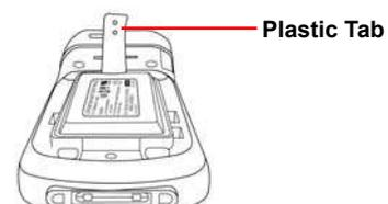
5. Replace the battery compartment cover by pushing down on the tabs and sliding them back into place as shown.
