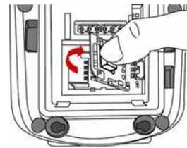
4. Insert the SIM card into the cover with the notched corner up, and the contact side of the SIM card faces down.
