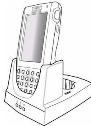
3. The connection is secure when the bottom edge of the device is aligned with the docking station, and the LED indicator on the device lights up red.
