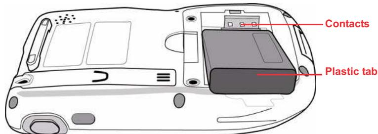
3. Slide the battery pack into the battery bay while simultaneously pulling the plastic tab and securing clip until the battery clicks into place.
