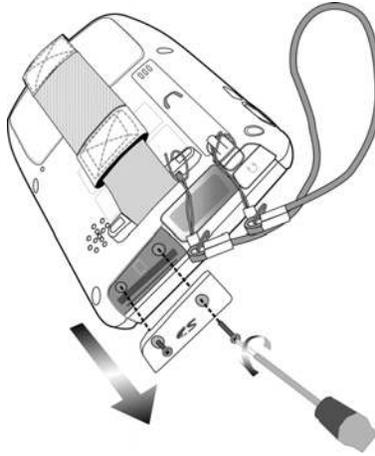
2. Insert the SD card with the notched corner as shown by the icon on the case.
