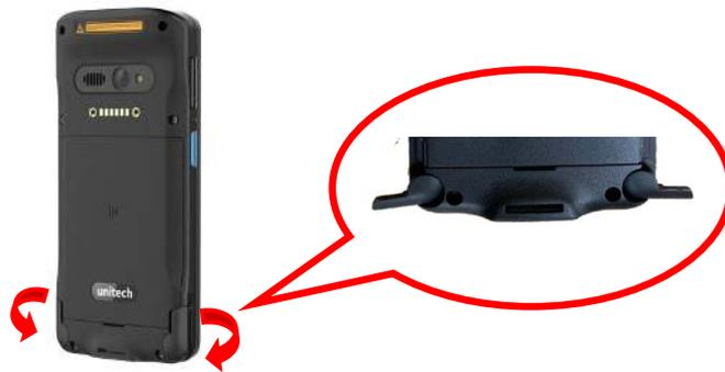
2. And pull the battery up to remove it.
