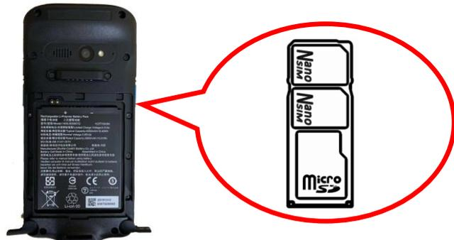
3. Put the battery back and lock the battery cover by turning the knobs a quarter of a turn (90°). Make sure the battery cover is securely closed, or you may be unable to turn on the terminal.
