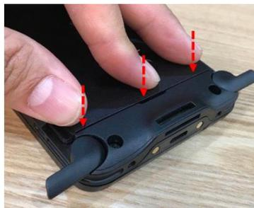
4. Lock the battery cover by turning the knobs a quarter of a turn (90°). Make sure the battery cover is securely closed, or you may be unable to turn on the terminal.
