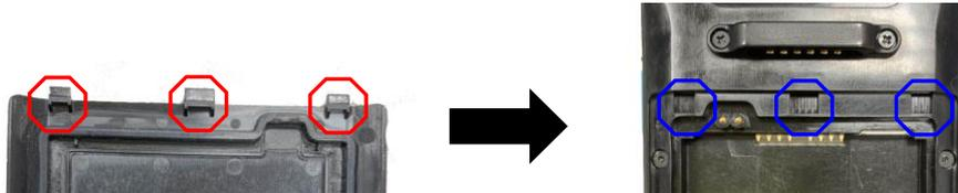
2. Insert the battery cover up to 45 degrees (45°), from top to bottom.
