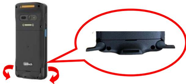
2. Remove the battery, and pull out the card slot.
