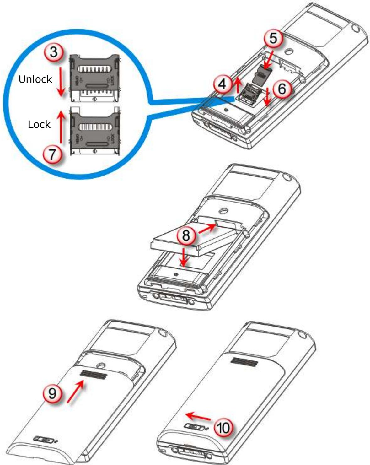
Figure 2: Installing the Main Battery & Memory Card
