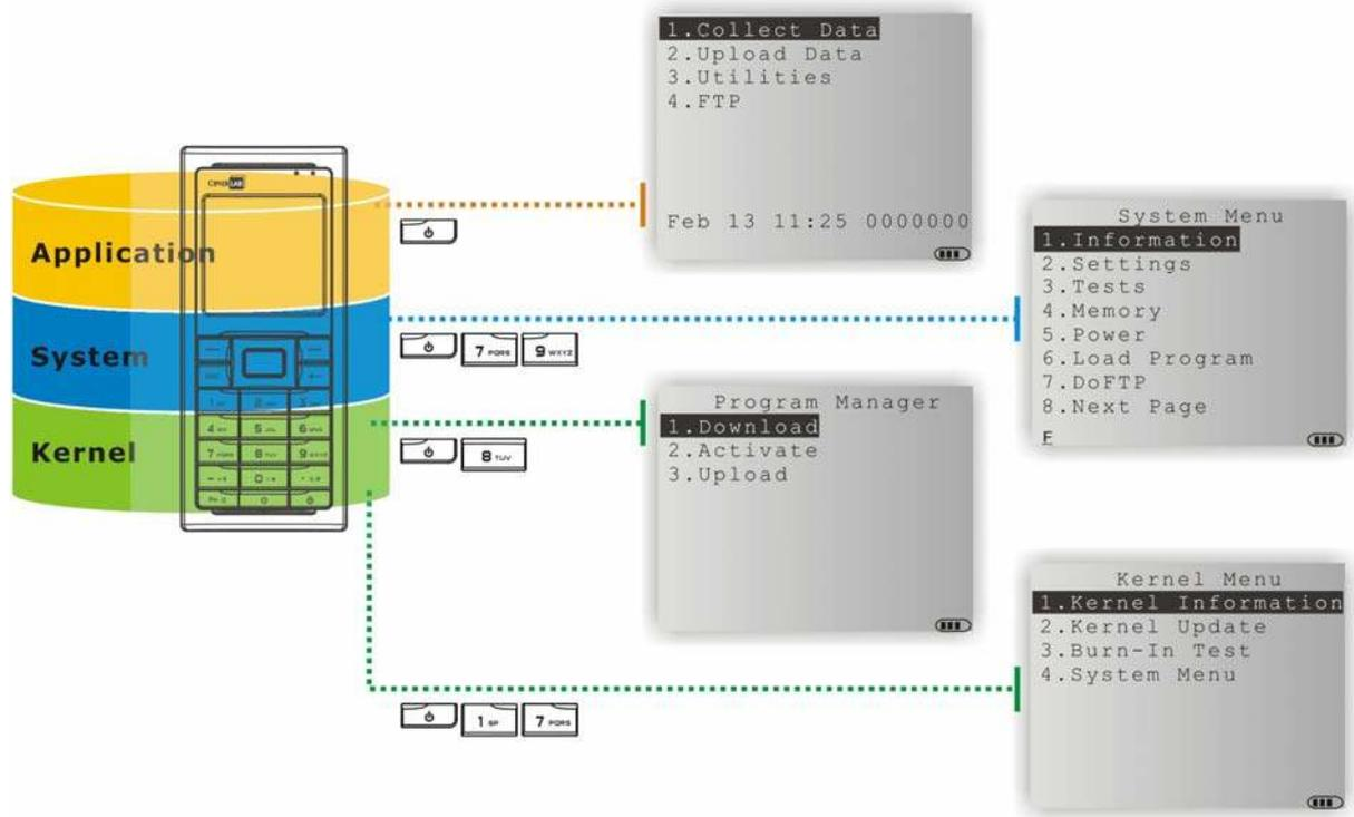
Figure 7: Software Architecture
